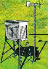
**Ground stations** hold instruments that measure air pressure, temperature, dew point, precipitation, wind speed, wind direction, and cloud cover.
